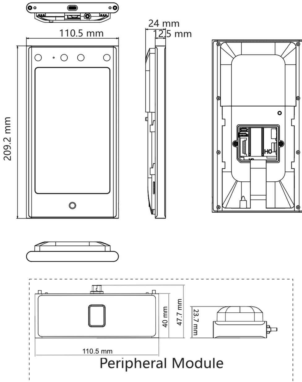
\*Notes: External modules are of same dimension. Here takes the fingerprint module as an example.
